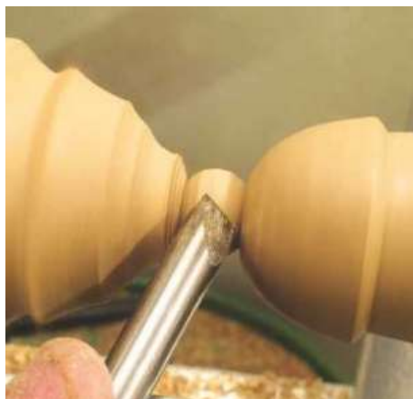
▲ Pic.29 The stem design is different from the pine prototype, and the ball is turned with the skew. Don't make the stem on the base too thin as it will not look balanced
